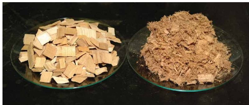
Figure 2. Photograph of untreated and steam-exploded mixed hardwood chips.
